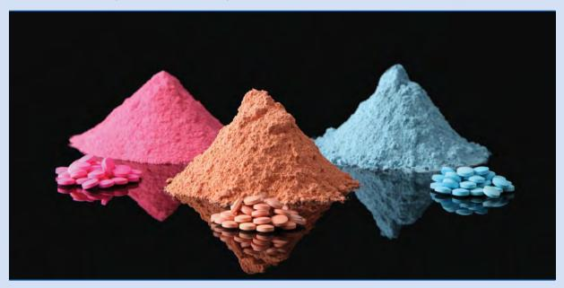
The color coats of the tablet (RT.FILM) are powder mixtures of polymers, plastisizer, pigments, antifoams, surfactants, anti-tacking agents and fillers. To coat the tablets, RT.FILM is dissolved at a specific concentration in water or alcohol and then sprayed on the tablets to form a uniform film with the desired thickness on the tablet core.
